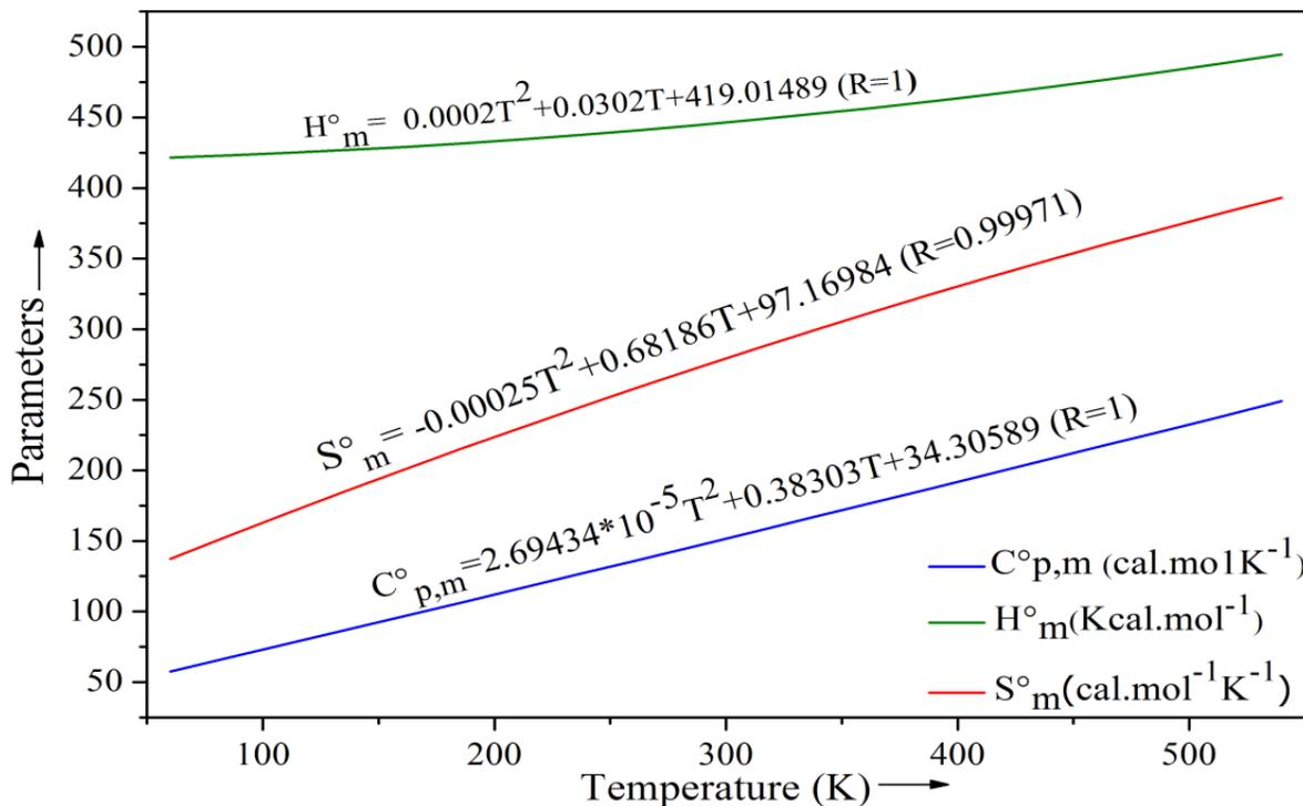
Figure 9. Correlation graphic of heat capacity ( $C^{\circ}p,m$  cal.molK-1), enthalpy ( $H^{\circ}m$  Kcal.mol-1), entropy ( $S^{\circ}m$  cal.mol-1K-1) and temperature for Coumarin doped BTCC
